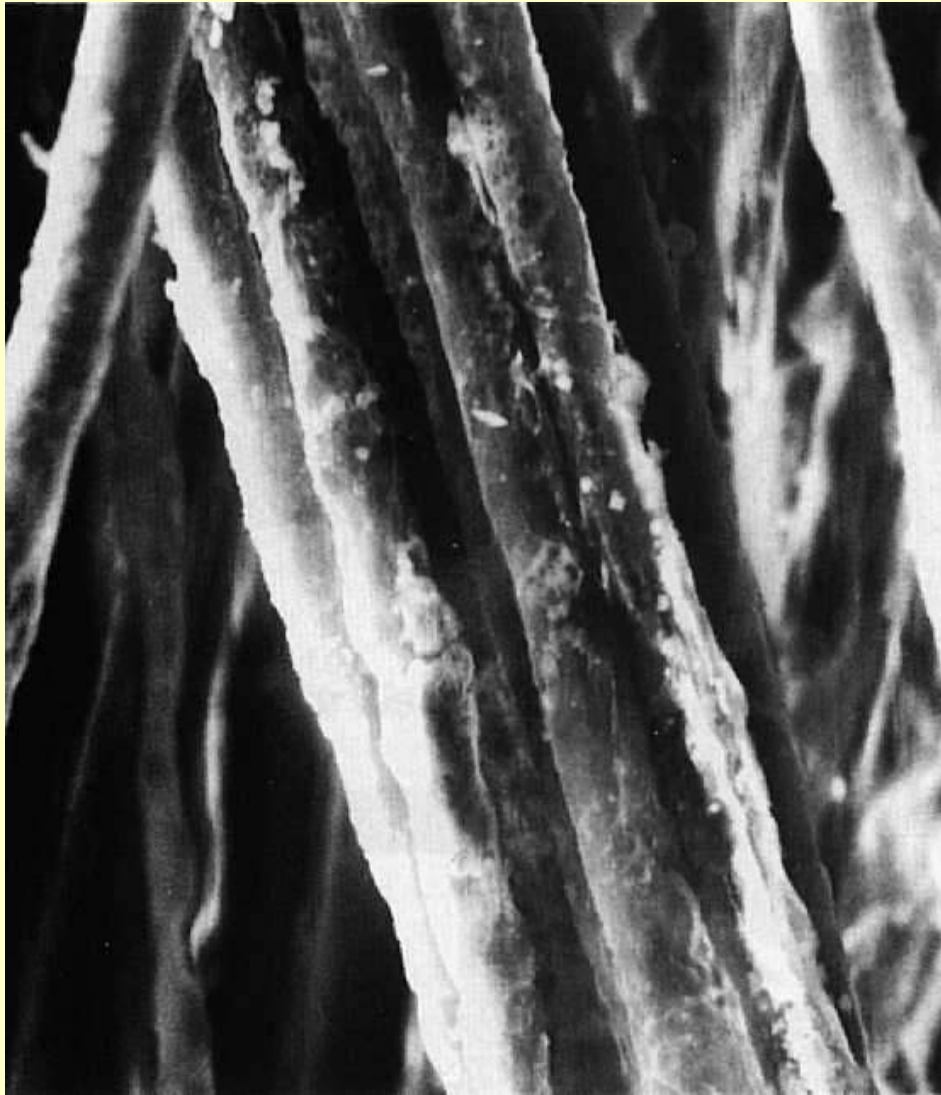
Scanning electron microscopy photomicrograph of Shroud's non-image fibers, showing the acrylic-polymer coating.
