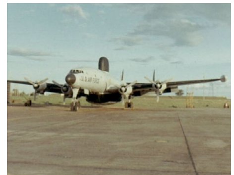
Left: The beam of the target tracking radar used to follow targets identified by the discriminating radar. 9 Right: An EC-121K "warning star" aircraft, like this one, optically tracked the incoming targets using visual and infrared wavelengths. 10
